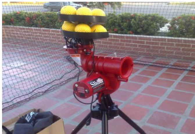
Fig -4: Batting practice ball launching system.
