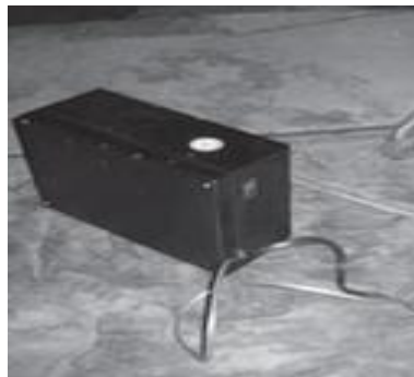
Fig -9: Control system used to turn on and off the piston before connecting it to the batting machine
