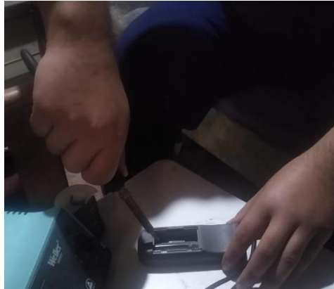
Fig -4: Soldering activity elaborated by worker (women), with incorrect method, generating stress and tired very quickly in the electronics industry evaluated (2023).
